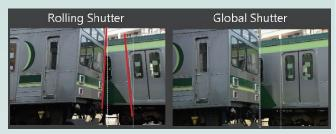
No Geometric Distortion with Global Shutter (Simulated images)
